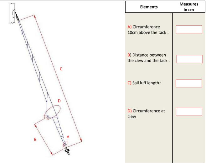
For measurement **D**: The circumference at the clew should be measured with the sheet knot as the cover will protect both.
